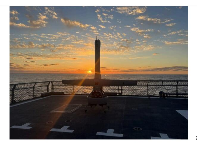
The V-BAT is the only single-engine, ducted-fan, vertical takeoff and landing (VTOL) UAS that is operationally deployed across multiple regions globally.
